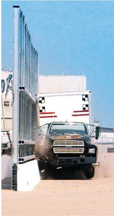
**The ACRYLITE® soundstop TL-4 System stabilizes the vehicle after impact**
